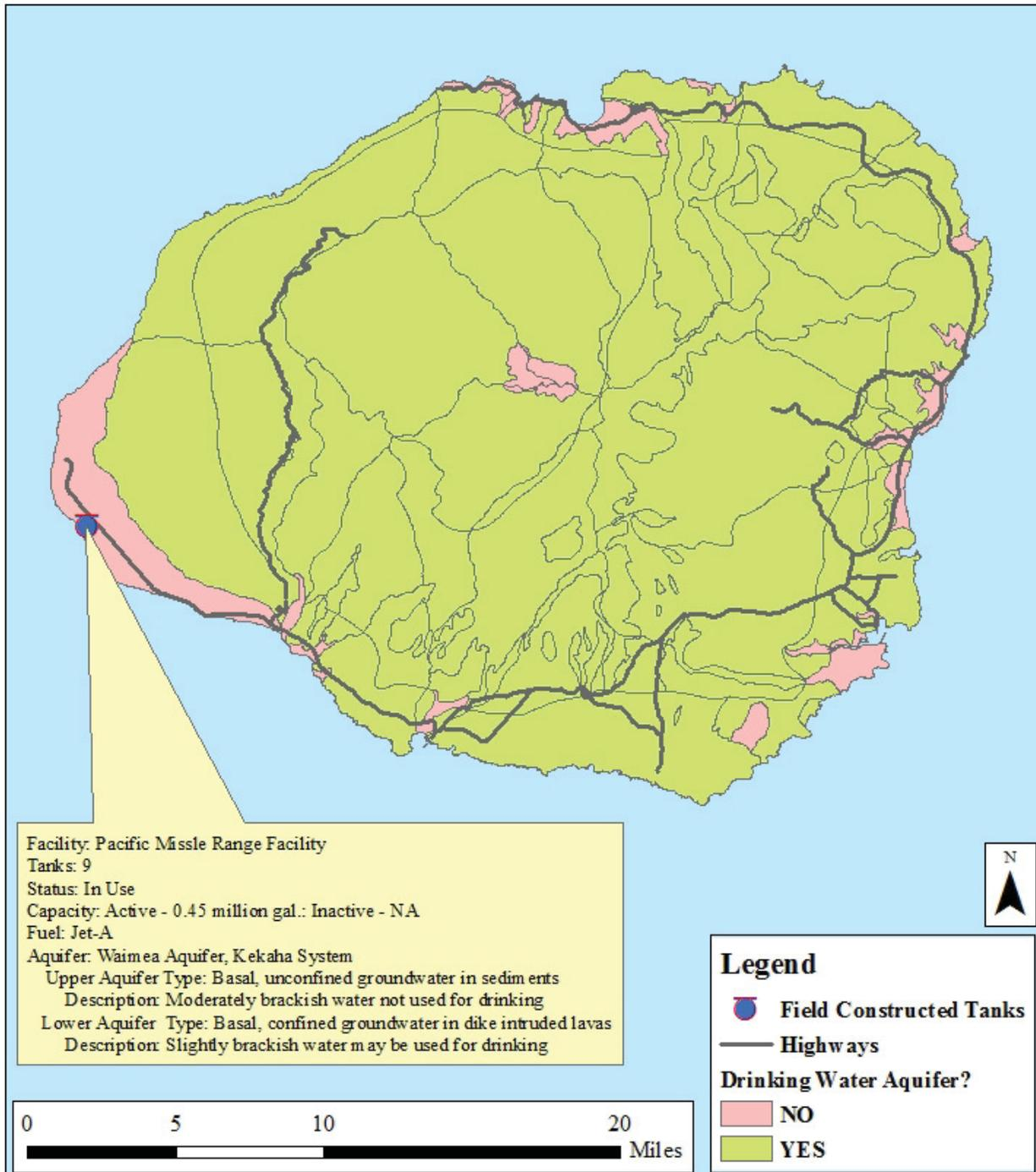
The Pacific Missile Range Facility is the only Hawaii location outside of Oahu where field constructed tanks are in service. The 9 tanks for this facility are located over a sedimentary aquifer that is not used for drinking water due to excessive salinity and low productivity. Below this sedimentary aquifer is confined groundwater that could potentially be used for drinking water. The potential drinking water aquifer is protected from contamination by the overlying sedimentary aquifer.
