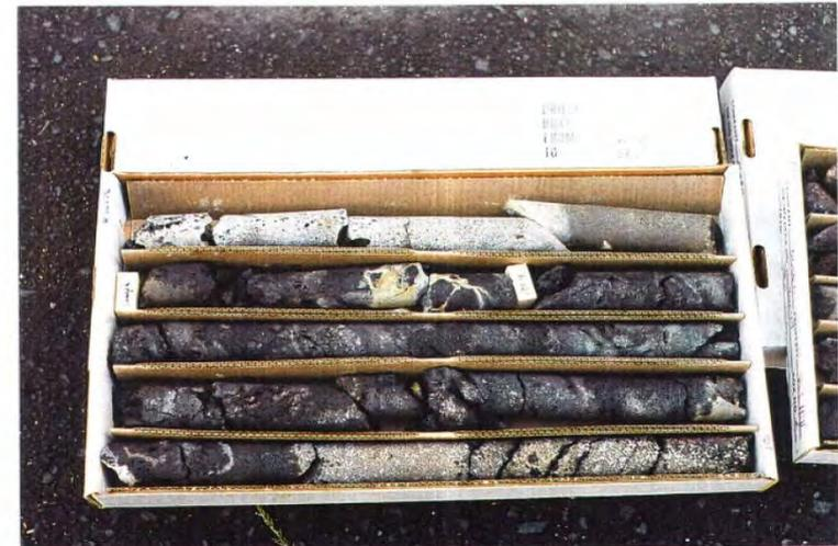
Figure 4-8 Petroleum Stained Core – B16C, 60' to 69'
