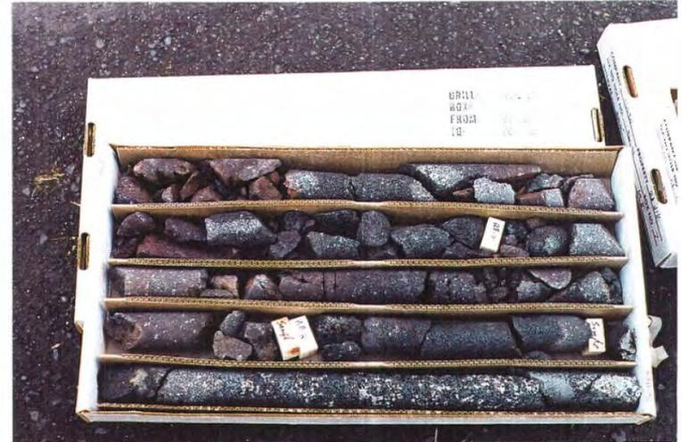
Figure 4-7 Petroleum Stained Core – B16C, 49' to 60'
