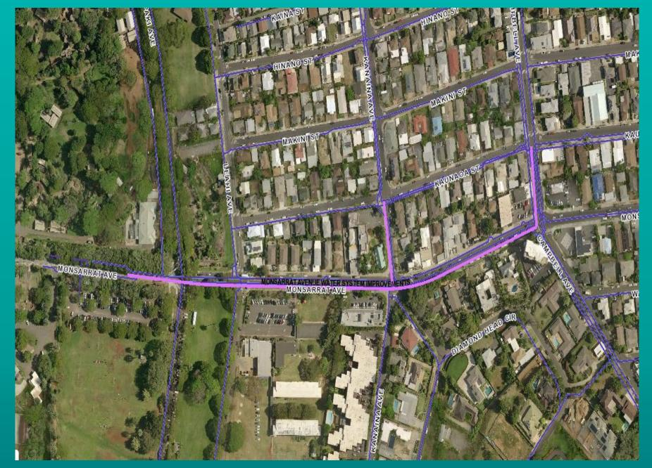
The Monsarrat Avenue WSI Project consists of existing cast iron 6-inch, 12-inch, 16-inch and 30-inch waterlines to be replaced with a new 24-inch ductile iron waterlines along portions of Monsarrat Avenue, Campbell Avenue, and Kanaina Avenue. These lines are recorded as constructed back as far as 1928 and has had several main breaks prompting the replacement of these segments.
