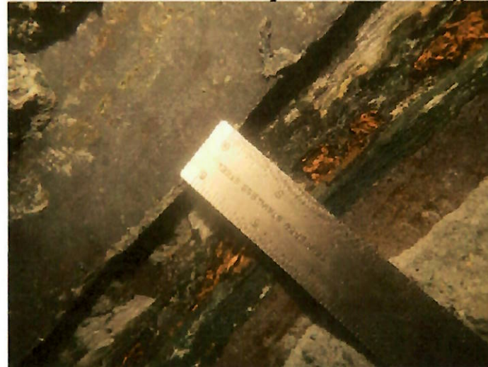
9 O'clock Position – 1-1/2" Separation, 1/16" Offset
