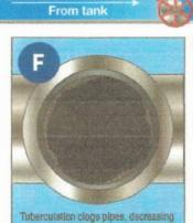
water pressure and negatively impacting distribution. Pipes that are regularly cleaned with UDF are safer, more efficient, and have a prolonged life span. UDF is one of the most cost-effective ways to maintain a safe, functional distribution system.
