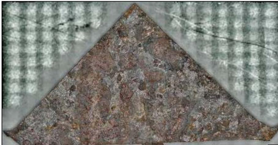
**Figure 176.** A screenshot of the 3D digital image of a specimen excised from Coupon A-1 labeled as A1-3, after CO<sub>2</sub> blast cleaning
