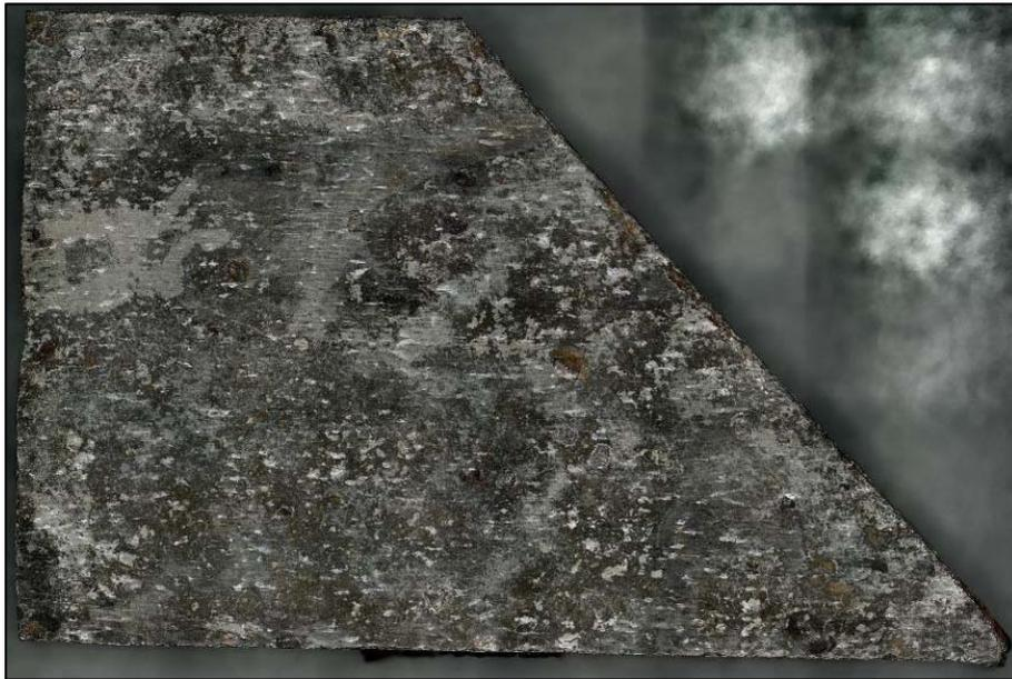
**Figure 173.** A screenshot of the 3D digital image of a specimen excised from Coupon 10 labeled as 10-3, after CO<sub>2</sub> blast cleaning
