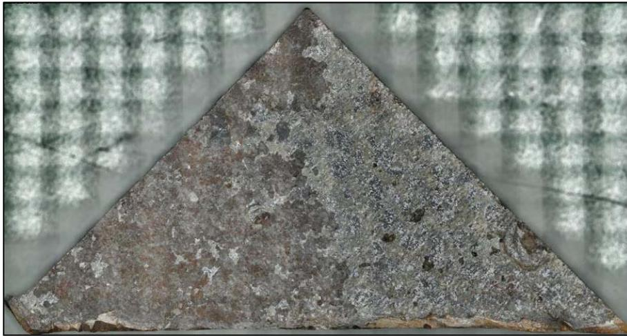
**Figure 169.** A screenshot of the 3D digital image of a specimen excised from Coupon 8 labeled as 8-2, after CO<sub>2</sub> blast cleaning
