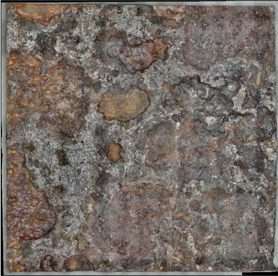
**Figure 165.** A screenshot of the 3D digital image of a specimen excised from Coupon 7 labeled as 7-2, after CO<sub>2</sub> blast cleaning.
