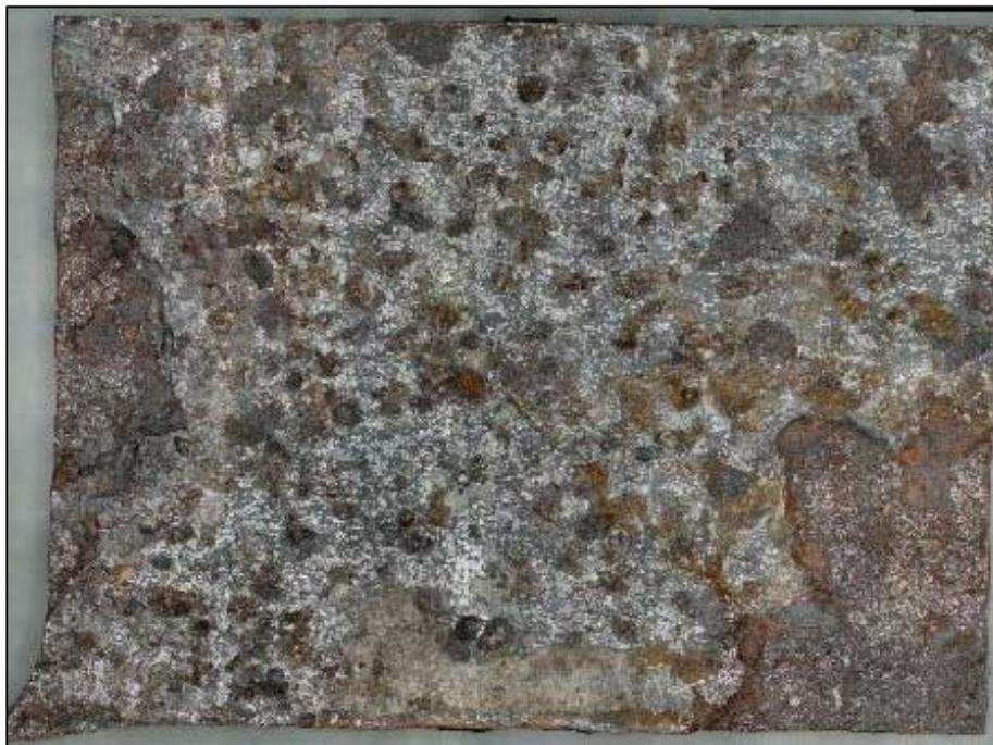
**Figure 174.** A screenshot of the 3D digital image of a specimen excised from Coupon A-1 labeled as A1-1, after CO<sub>2</sub> blast cleaning
