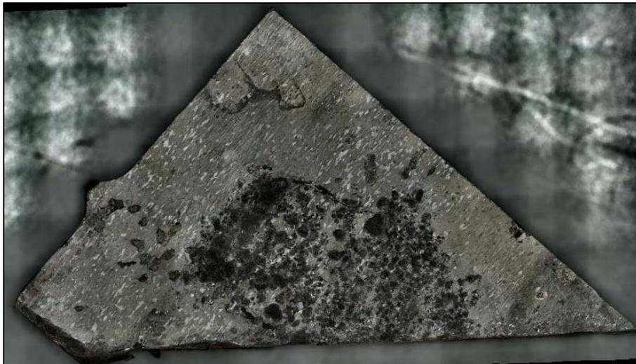
**Figure 172.** A screenshot of the 3D digital image of a specimen excised from Coupon 10 labeled as 10-2, after CO<sub>2</sub> blast cleaning
