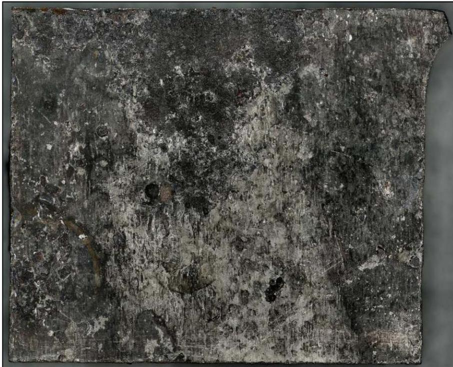
**Figure 171.** A screenshot of the 3D digital image of a specimen excised from Coupon 10 labeled as 10-1, after CO<sub>2</sub> blast cleaning
