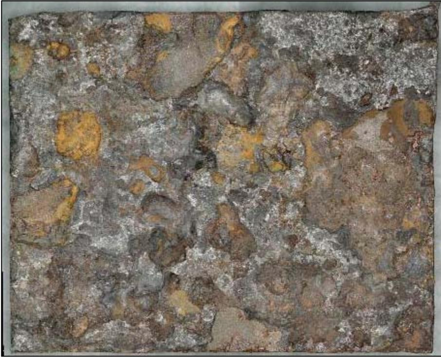
**Figure 166.** A screenshot of the 3D digital image of a specimen excised from Coupon 7 labeled as 7-3, after CO<sub>2</sub> blast cleaning
