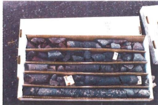
Figure 4-7 Petroleum Stained Core - B18C, 49' to 60'
