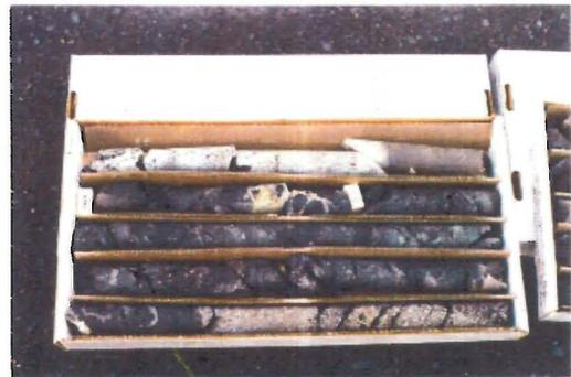
Figure 4-8 Petroleum Stained Core - B18C, 60' to 65'
