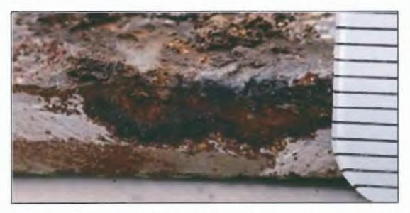
Figure A-5. The same area is shown in an image provided prior to shipping Coupon #7 to IMR (provided to IMR on March 13, 2019). What appeared to be a deep corrosion pit was actually rust-colored staining of the edge surface
