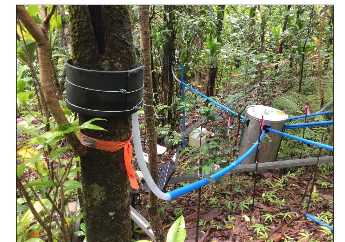
Stemflow Equipment: Stemflow collectors connected to a fabricated tipping bucket (150 mL / tip) rain gauge were used for each test plot. Trees selected for stemflow data collection represented the range of typical species, diameter and height found commonly on the test plots. Stemflow collectors were supported through lengths of 7/8-inch diameter poly tubing protected in 1-inch diameter HDPE pipe, leading toward the rain gauge, nested in a stainless steel can, levelled and anchored.
