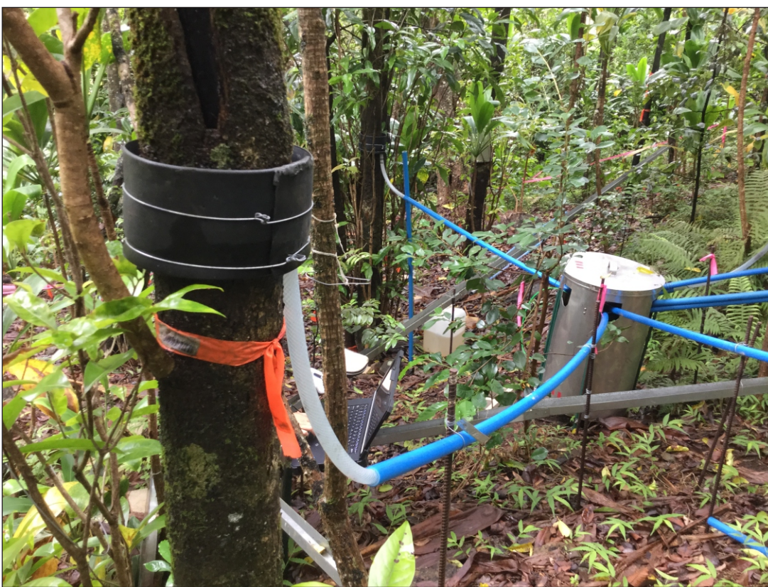
Stemflow Equipment: Stemflow collectors connected to a fabricated tipping bucket (150 mL / tip) rain gauge were used for each test plot. Trees selected for stemflow data collection represented the range of typical species, diameter and height found commonly on the test plots. Stemflow collectors were supported through lengths of 7/8-inch diameter poly tubing protected in 1-inch diameter HDPE pipe, leading toward the rain gauge, nested in a stainless steel can, levelled and anchored.
