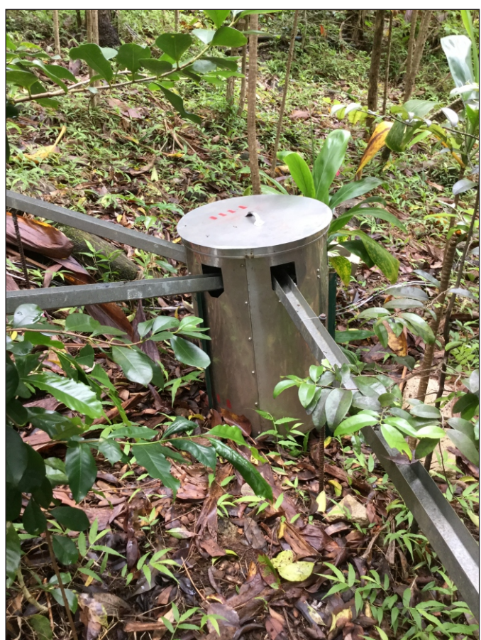
Throughfall Equipment: For each test plot, a total of three troughs lead to a fabricated tipping bucket (150 mL / tip) rain gauge. The gauge is nested in a stainless steel can, levelled and anchored to the ground for stability. Troughs were installed under trees typical of the test plots (species, diameter, height) in configurations that represented the average canopy and gap proportions and minimized overlap of throughfall collection between troughs.
