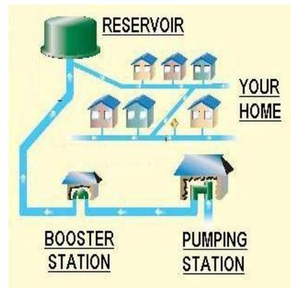
As you can see, the freshwater flowing from your tap is the result of a long and complicated process. For more information on our water supply or the BWS Transmission System, visit [www.boardofwatersupply.com](http://www.boardofwatersupply.com).
