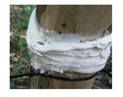
Silicone- made for wet conditions/ waterproof, but Has a long cure time. It is difficult to create a thick, smooth surface.
