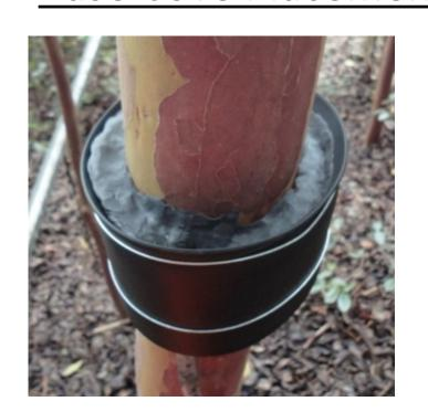
It is important to place the base cove high enough around the duct seal to create a reservoir to allow the collected stemflow time to drain into the tubing. The picture shows the base cove placement too low on the duct seal. There is no reservoir, and water can run off the top of the collar draining into the tubing.
