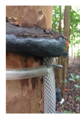
If wire is used to secure the tubing to the tree, the tubing should be checked a few times a year to ensure the tubing is not compromised as the tree grows. Disturbance to the duct seal may lead to leaks and the collar may need to be redone.
