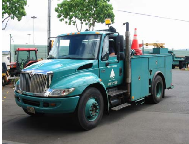
Diesel Retrofits. BWS trucks were retrofitted with devices that burn off and filter out much of the diesel particulate matter before discharging it.
